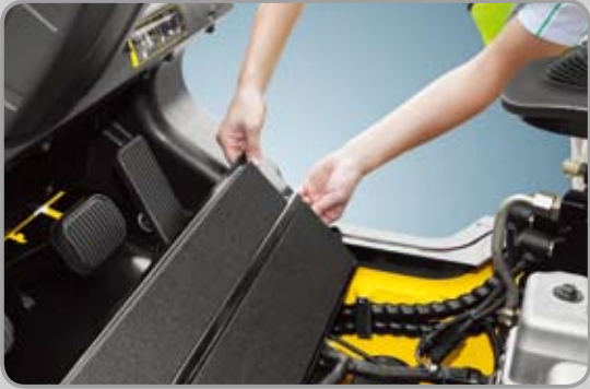
Tool-less floor plate for serviceability.
